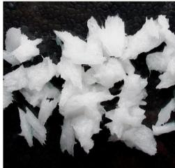
The creation of the latent heat blended material RUBITHERM® SP has led to a new and innovative class of low flammability PCM. RUBITHERM® SP consists of a unique composition of inorganic components.
